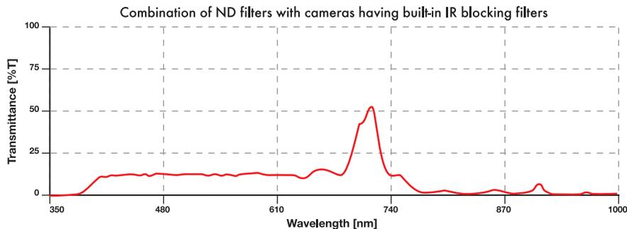
For this purpose, Tiffen pioneered the **Full Spectrum IR ND Filters** designed to provide a true neutral density into the IR spectrum to correct this issue. Tiffen’s Full Spectrum IR ND Filters now allow for the use of heavier grades of Neutral Density filters needed for these hi-definition cameras while, at the same time, maintaining color balance.
